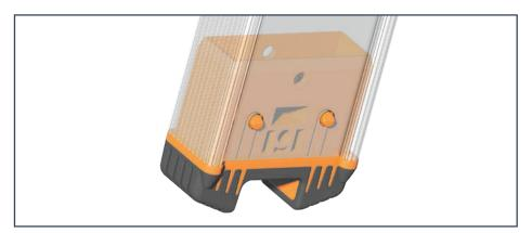
The Layher Combigrip ladder foot is made of a 2-component plastic: a hard inner section (orange) for secure mounting inside the stile, and a soft outer covering (black), non-slip on every floor surface. That ensures:
