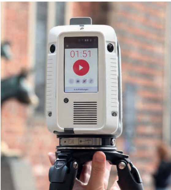
The scanner needs just under two minutes to complete one run.
