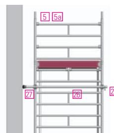
For work performed on a load-bearing wall, ballasting can be reduced in accordance with the ballasting table (see p. 7).
